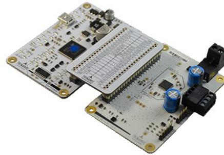
Figure 3: TMC5130A-TA evaluation board
