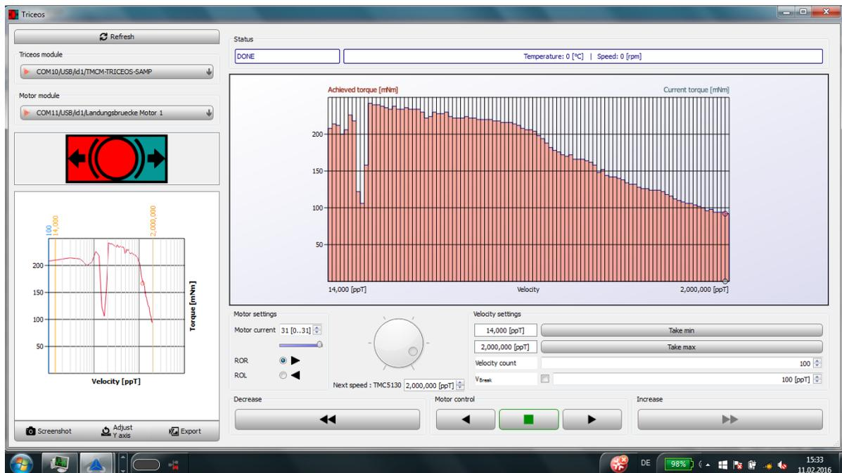
Figure 4: View of motor test rig GUI after one complete test series
