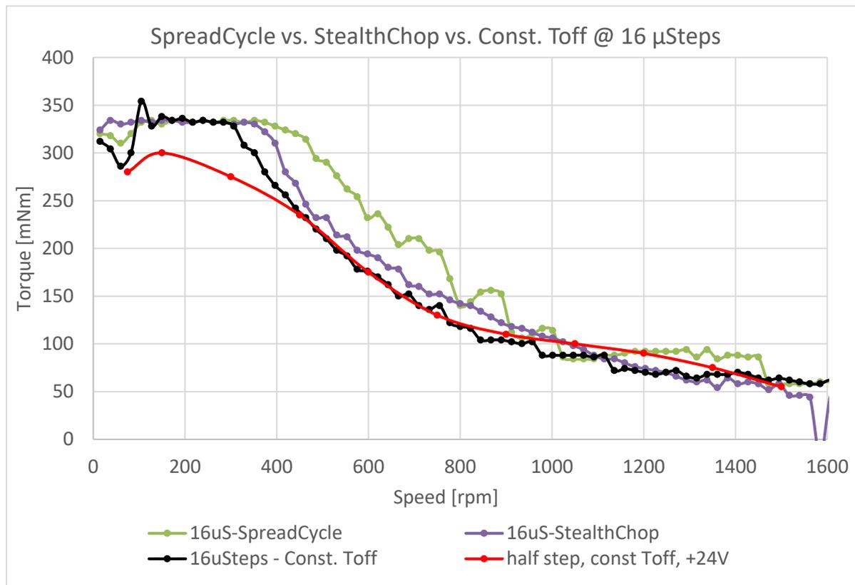
**Figure 7: Torque/speed chart with comparison of three chopper modes @ 16µSteps**
