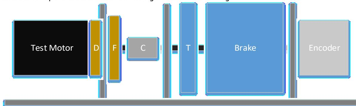
Figure 1: Principle architecture of the motor test rig
