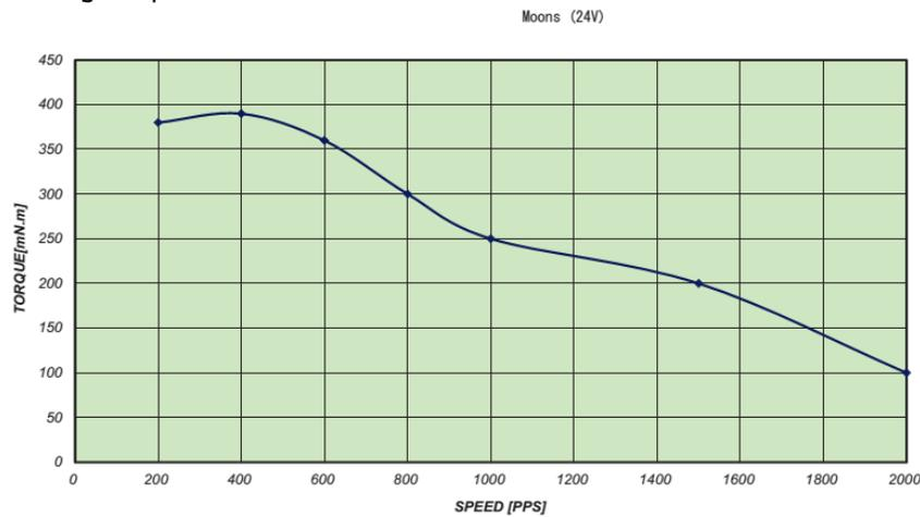
**Figure 9: Manufacturer's pull out torque diagram (@ 24V, constant Toff, no dampening, full step operation, 200pps = 60rpm, 1000pps = 300rpm, 2000pps = 600rpm)**
