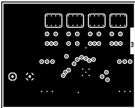
Figure 6: Inner layer (GND)
