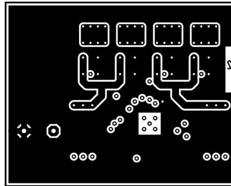
Figure 5: Inner layer (Supply)
