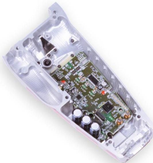
*Figure 1 – Miniaturized PCB custom-made for a perfect fit in Össur’s Power Knee, a battery-powered prosthetic leg.*
