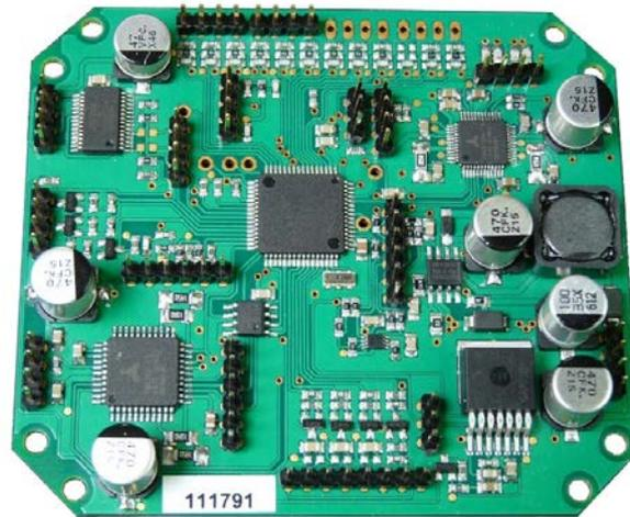
Figure 14 - The controller PCB for the electromechanical actuators of the tangential tonearm DTT-01-S, along with Trinamic's smart stepper motor driver solutions. (Courtesy of AVDesignHaus)
