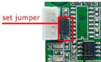
Figure 4.8: Jumper for placing bus termination
